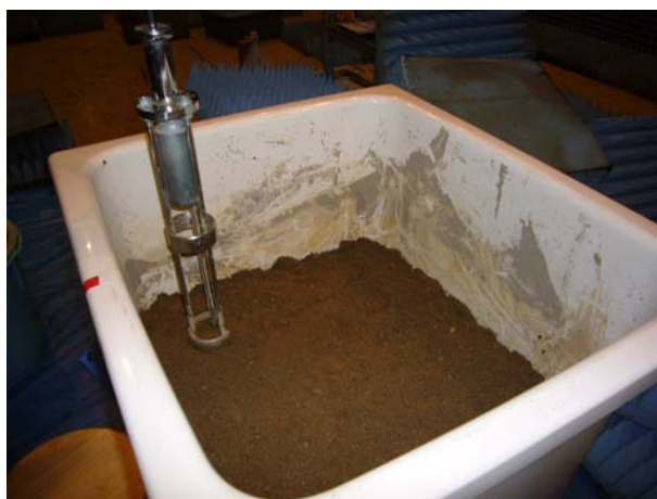
Figure 1: Soil specimen after compaction was completed
