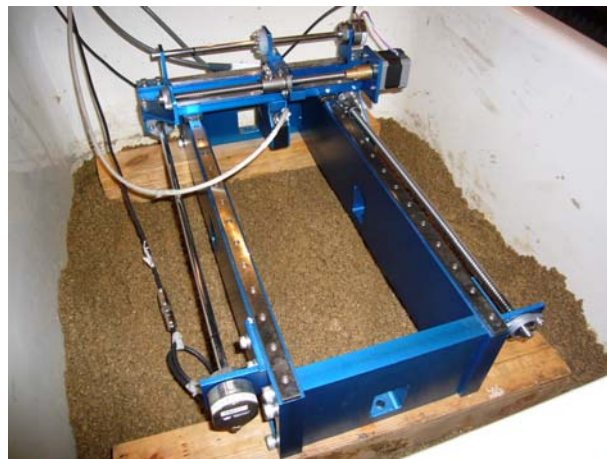
Figure 2: Measurement of soil surface roughness by laser scanner
