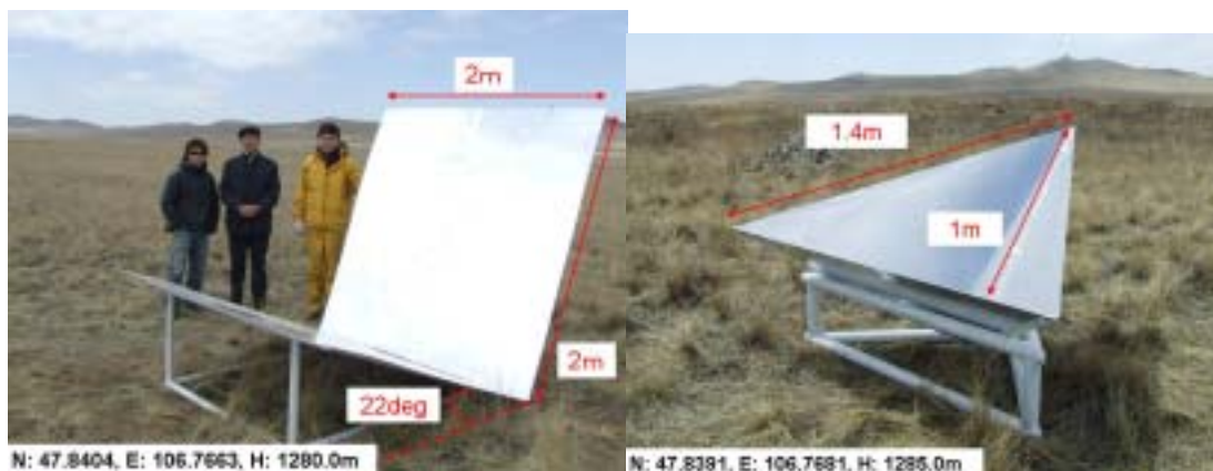
(a) Dihedral Corner Reflector (b) Trihedral Corner Reflector Figure 2 Corner Reflectors
