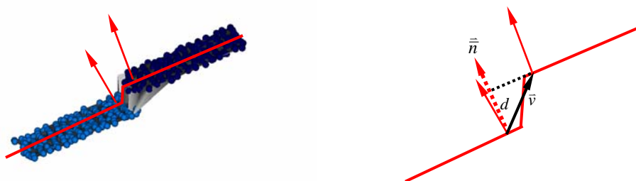
Figure 6. Segmentation of two neighboring planes with the same normal vector by a height difference condition
