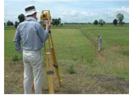
Figure 2: Measurement of surface roughness (No. 4 in Table 2)
