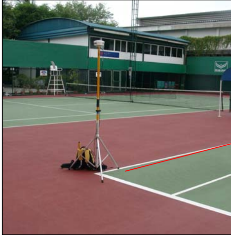
Figure 3.2.5 Tennis court corner, GPS observation.
