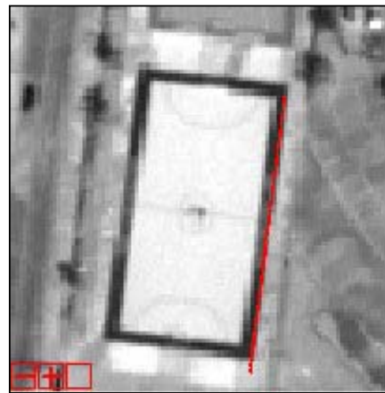
Figure 5.4 A linear feature collected using Kinematic GPS observation method (DGPS corrected), overlay after geometric correction of the image.
