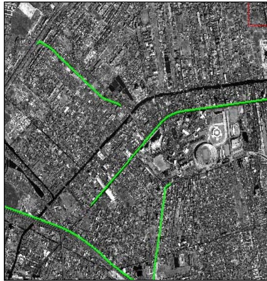
Figure 5.2 The four long linear feature collected using Kinematic GPS observation method.
