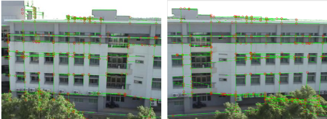
Fig. 3: Detected lines and their intersection points.
