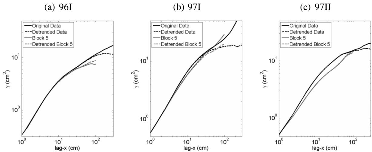
Fig 5: Original data is referred as the large sampling size (6m x 6m). Block 5 is the small sampling size (2m x 2m) at the center. Detrended parameters of block 5 used the same parameters applied for detrending the large sampling area.
