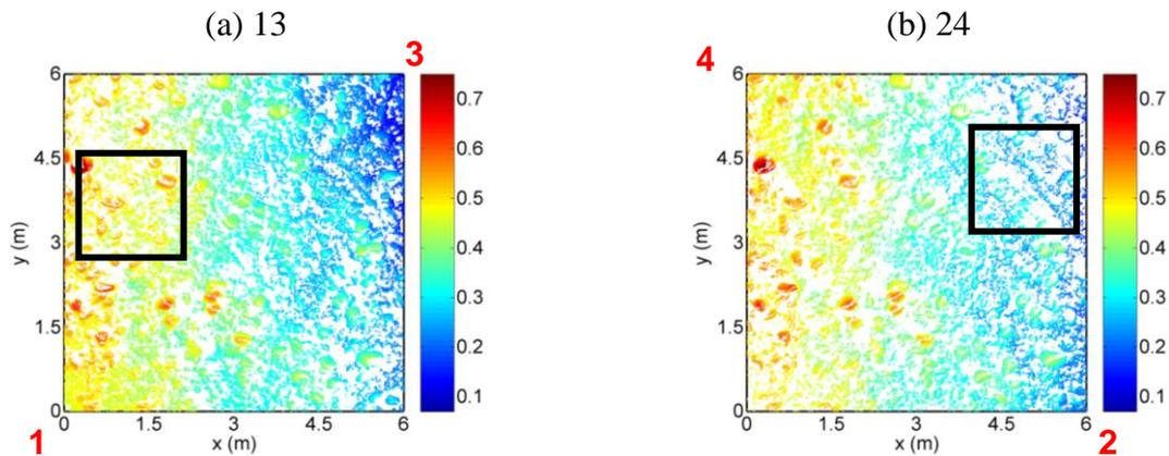
Figure 7: The DEMs of lidar station arrangement 13 and 24 in site 97I. The red number denoted the position of lidar station. The black rectangle denoted the shadowing effect.
