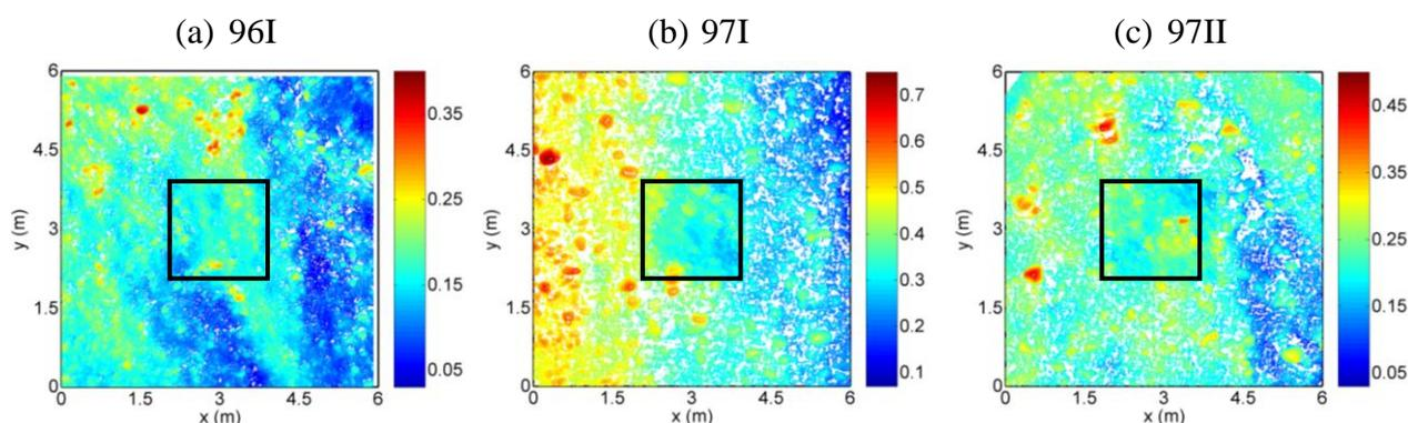
Figure 4: Digital elevation models of three sites. The black rectangle represented the small patch size (2m x 2m). The coverage of site 96I, 97I and 97II was 93.23%, 73.41%, and 80.65%, respectively.
