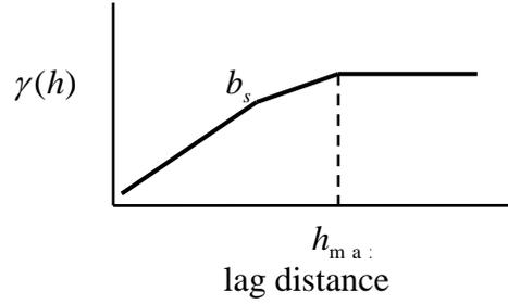
Figure 1: Statistical properties of gravel bed profiles on log-log scale. The break of slope  $b_s$  identified two different roughness characteristics at different scales. The range of the variogram is denoted as  $h_{\max}$ , which implied no spatial dependence is found after  $h_{\max}$ .
