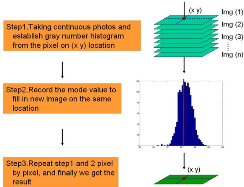
Figure 3. The flowchart of the mode-based filter.
