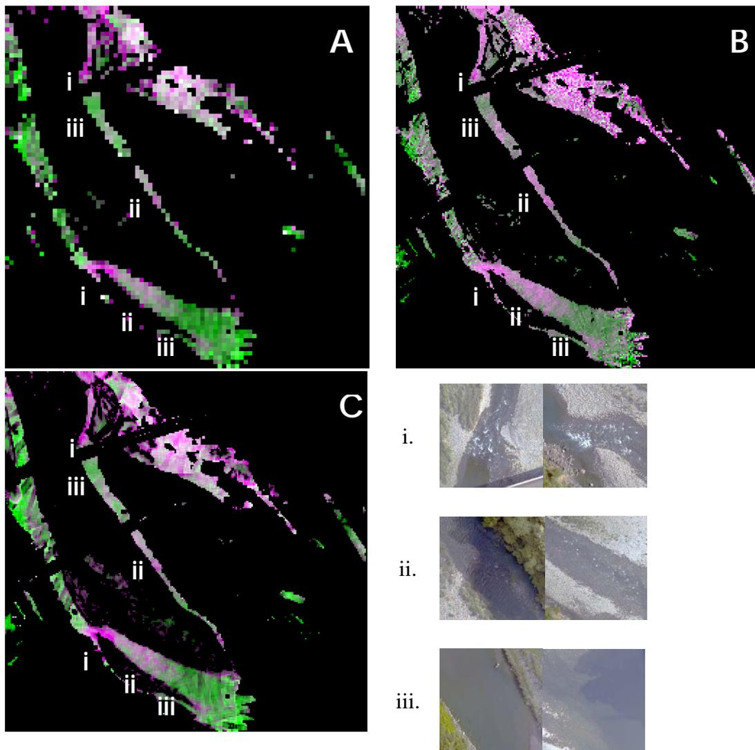
Figure 4. False color images (after masking). R: PC1; G: PC2; B: PC1. (a) 6 m x 6 m window size with 6 m stepping distance. (b) 2 m x 2 m window size with 2 m stepping distance. (c) 6 m x 6 m window size with 2 m stepping distance. Typical conditions of (i) BSW, (ii) USW, and (iii) NP in orthophoto.
